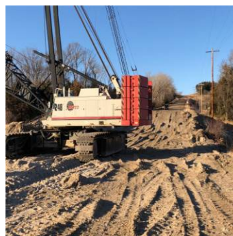
11/15/20 Looking north. Counter weights on the crane equal 83 Ton.
